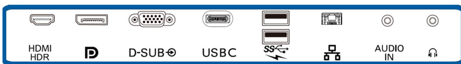
I/O back panel connector diagram
